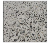
CON-01 Location / Floor Product: Concrete Finish: Polished Concrete Colour: Light Grey w/ Black Aggregate Code: - Note: Treated Floor Slab on Structural Steel Decking
